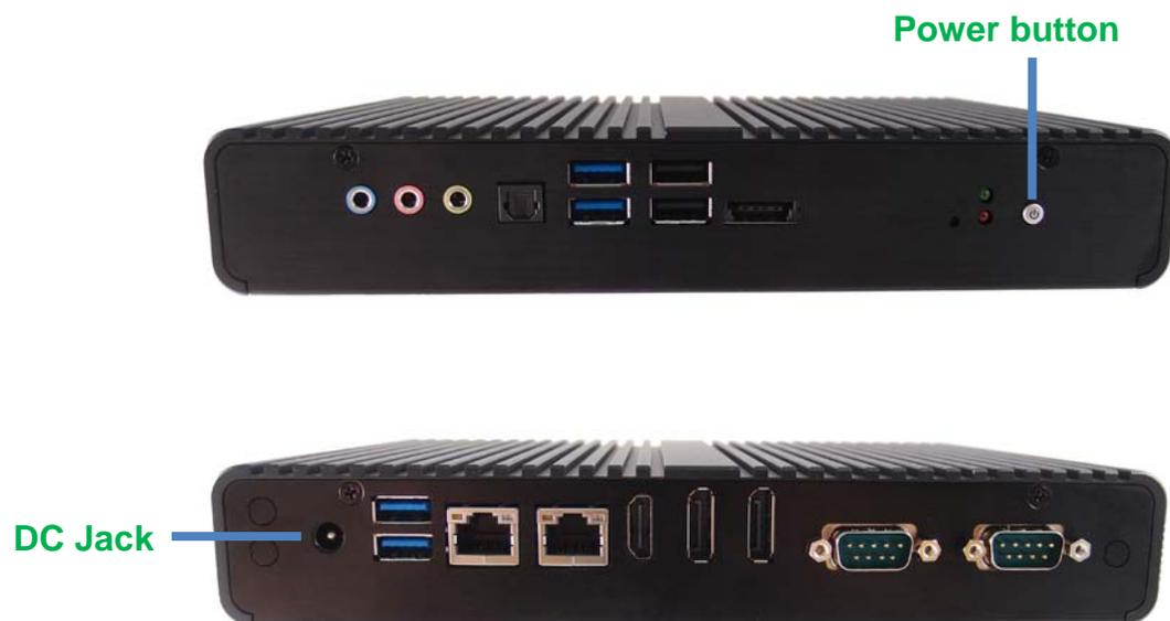
*Figure 8 Turning on the system*
