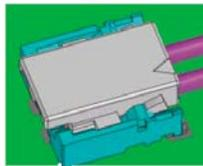
Push down to insert the cable side
