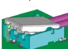
Continue lifting, the reinforced lock is released
